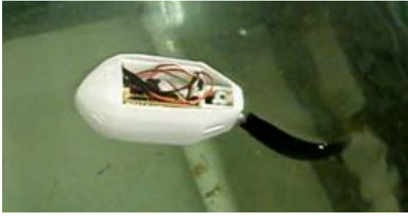
Figure 1: A prototype 3D-printed robotic fish with a flexible caudal fin.
